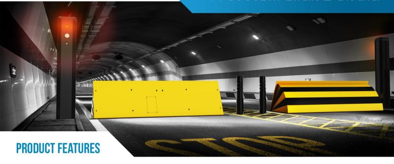
The PF8000SM road blocker has been designed for easy installation with minimal ground works required. This shallow mounted blocker is driven via a hydraulic pump power pack with inverter/plc controls requiring a single phase supply.
